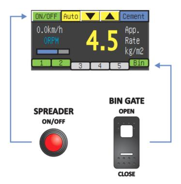
The screen shows figures for vehicle speed in km/hr, rotor speed in RPM (revolutions per minute), a horizontal bar graph representing the state of the hydraulic proportional valve from fully closed to fully open, and selected application rate in kg/m2. If the rotor RPM goes above 45 RPM the power light flashes on and off and screen flashes red indicating operational limit has been reached. The application rate and/or vehicle speed should be reduced accordingly.
