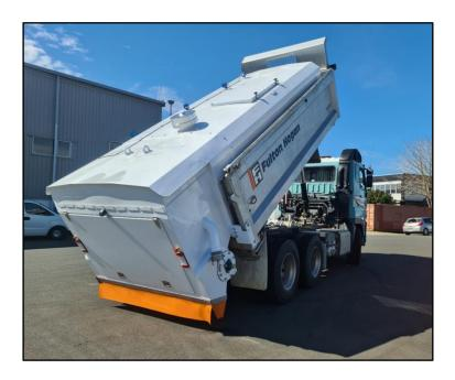
The unit provides for easy transfer from cement to lime or other spreadable material and utalises customer presets for quickly changing setups.
